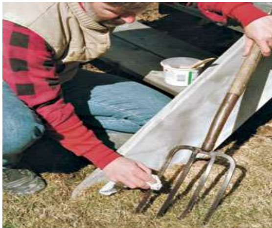
Fig.2 Oil steel tool heads to prevent them from oxidizing.
