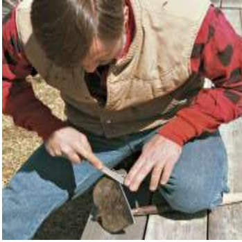
Fig.6 Use a hand-held mill file to sharpen hoes and shovels. The key to successful sharpening is Keeping the tool steady and the file at the proper angle.
