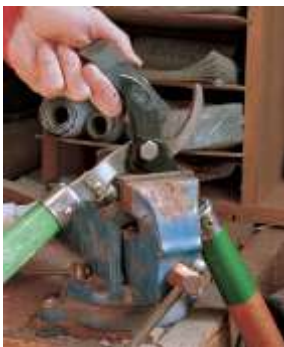
Fig.7 Sharpen pruning blades and knives by sliding an oiled honing stone in one direction across the tool's beveled edge.
